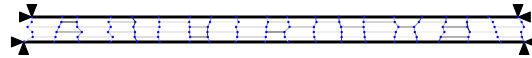
Fig. 15. Optimal core topology for the broadband case. The frame shading level code of the core from white to black describes the thickness variation from 0.32 to 4.41 cm.
